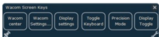
Screen Key panel: A Screen Key panel is a row of buttons that displays in the layout you choose.
