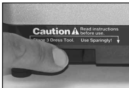
Figure 15. Use dressing tools sparingly.
