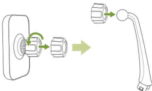
2. Insert the ball end of the arm into the fitting on the back of the desk mount and tighten the collar around the fitting to secure the arm.
