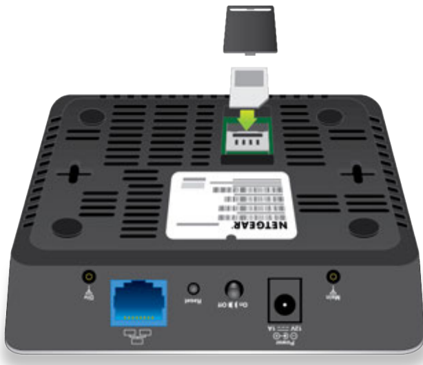
Figure 2. Overview of installing the micro SIM card
