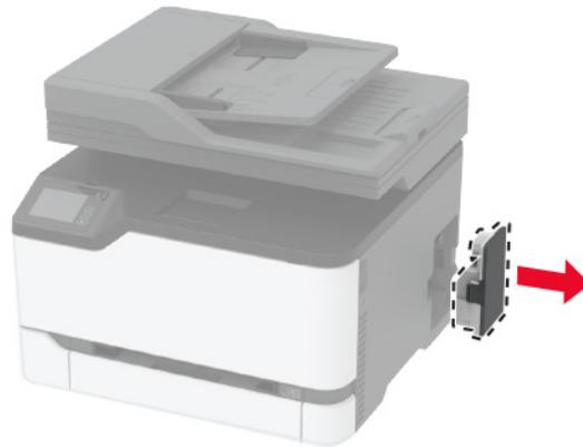
**Note:** To avoid spilling the toner, place the bottle in an upright position.
