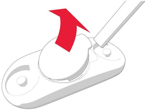
2. Remove the old battery from the battery cover.
