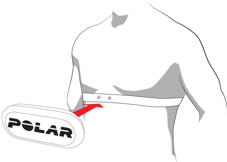
**i** Detach the connector from the strap and rinse the strap under running water after every use. Sweat and moisture may keep the electrodes wet and the heart rate sensor activated. This will reduce the transmitter battery life.
